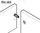
Tighten the cam lock screw **X**Use Allen Key or Screwdriver
